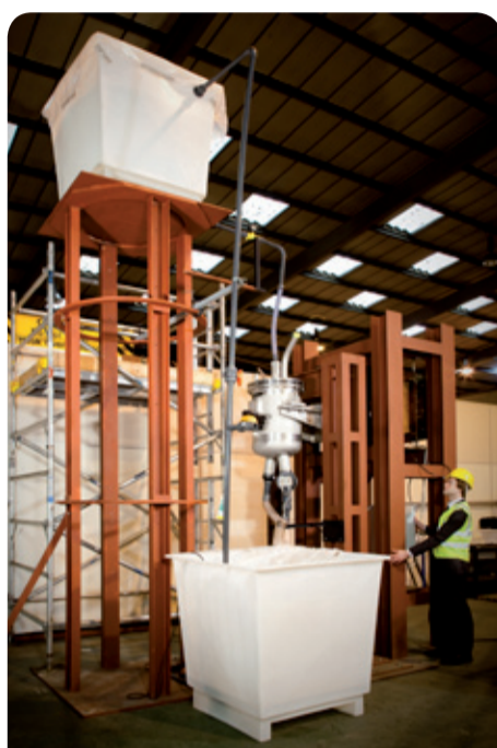
A specially designed rig was used to test the equipment using a water load.
