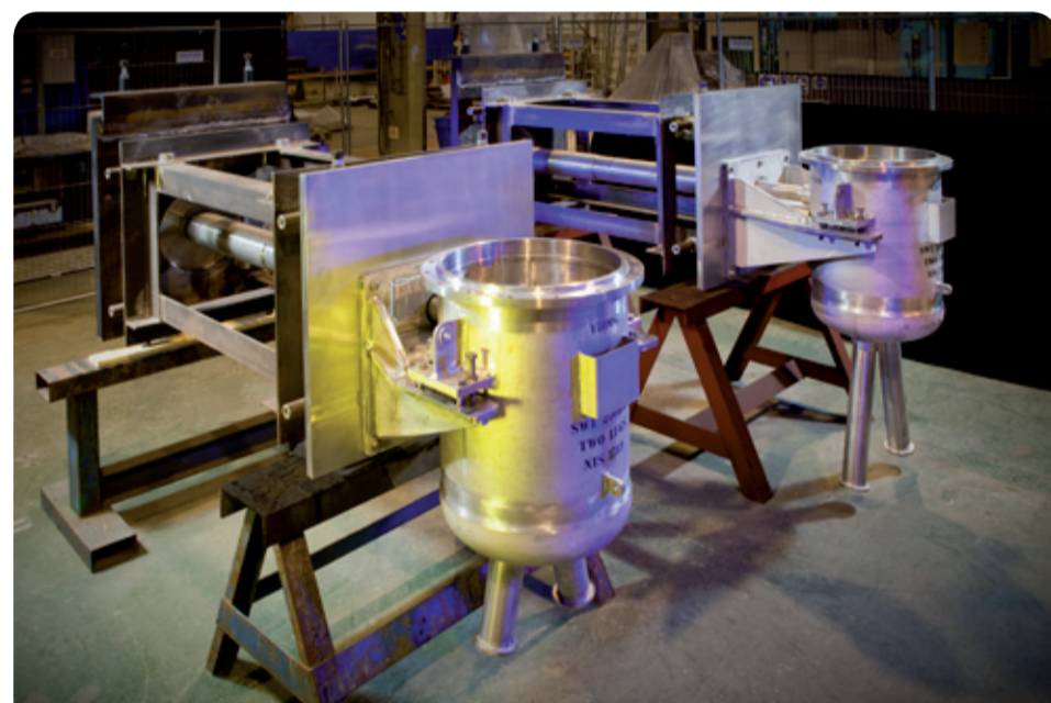
Manufacturing the vessels involved complex fabrication and high integrity welding.
